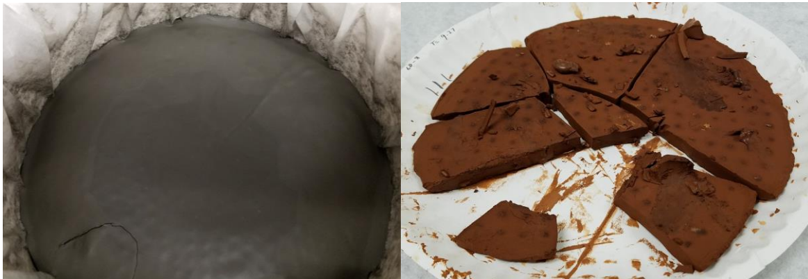
Figure 1 Comparing original sulfide floatation concentrate to post AAO process oxidized concentrate that is readily leachable with standard CIL gold extraction.
